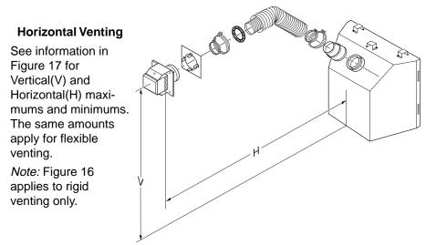
Figure 18 - Horizontal Termination Using Flexible Venting
